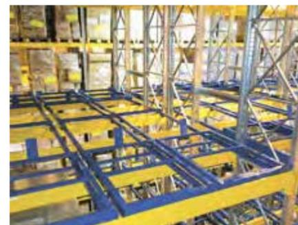
Push-back shelving is an accumulation storage system that allows you to store up to four pallets in depth per level.
