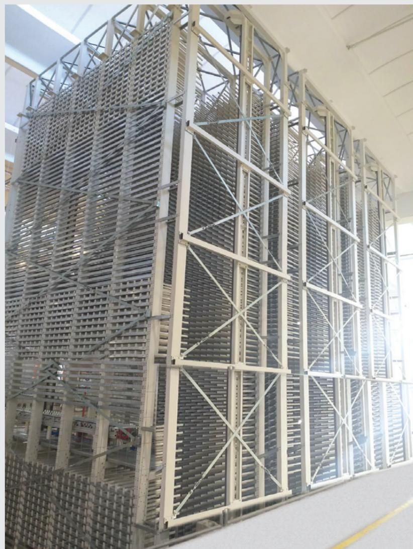
The automatic warehouses for bars and long bodies have been designed to best manage and store items characterized by a considerable length, while exploiting the available height at the same time.
