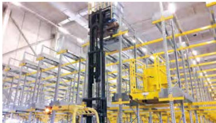
**SAT DRIVE** Storage system for pallets high density in which the loading and unloading of the goods is facilitated by the radio-electric shuttle called radio-shuttle. The latter moves autonomously inside the tunnels of the shelving, without requiring the entry of forklifts. The operator guides all the movements of the storage and retrieval in a simple way via a radio control.
